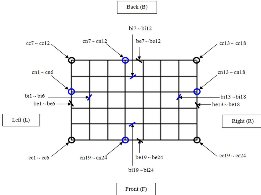
Figure 6. Plan view of building with locations of selected members ( $\alpha_0 = 0^\circ$ )
