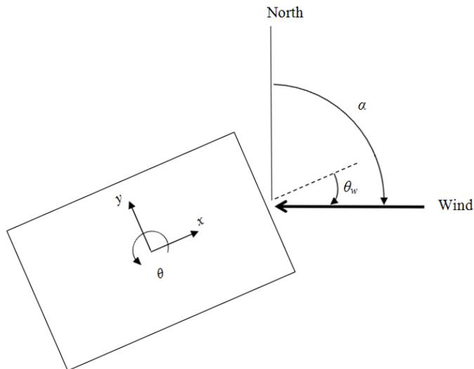
Figure 5. Local coordinates of the building and wind directions
