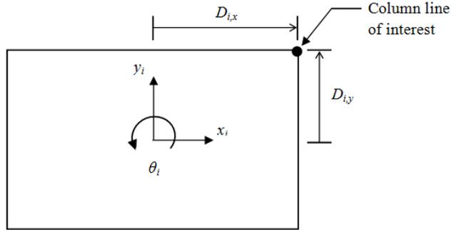
Figure 2. Position parameters at floor  $i$  for interstory drift ratio
